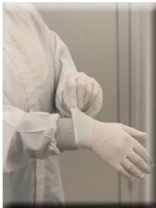
**9** Roll down donning gloves slightly to expose cuff. Snap cuffs of coverall (if applicable). Place cleanroom working gloves over or under the cuff depending on your requirement.
