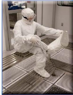
**2** Remove goggles. Remove boots one at a time without letting the tops touch the step or floor areas.
