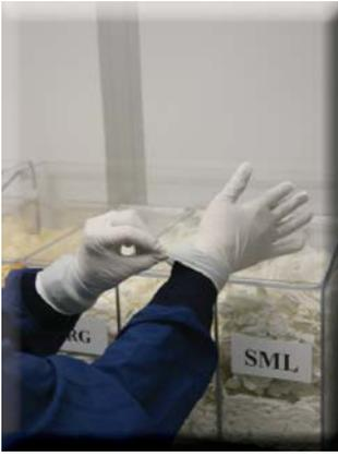
**1** Don two pairs of cleanroom gloves, placing the second pair over the first pair.
