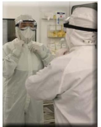
**12** Use a mirror to check proper gowning. Discard donning gloves and enter the cleanroom.
